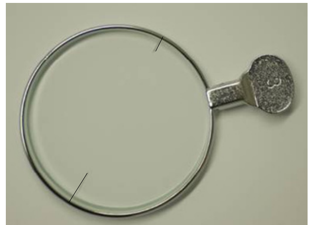
Figure 8.8: Metal rimmed prism trial lens. This lens is a 3 rd prism. It has a small line at the apex of the prism, and a longer line at its base. You must be extremely careful not to confuse prism and cylindrical trial lenses.
