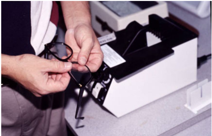
Figure 27.7: Using a frame heater to adjust a plastic spectacle frame
