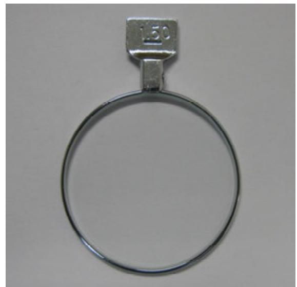
Figure 8.3: A metal rimmed spherical trial lens. The power of the lens is written on the lens. This is a -1.50 D trial lens.
