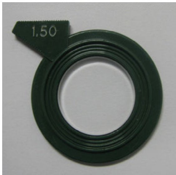
Figure 8.2: A plastic rimmed spherical trial lens. The black colour tells you that it is a plus lens, and the number tells you the power. This is a +1.50 D trial lens.
