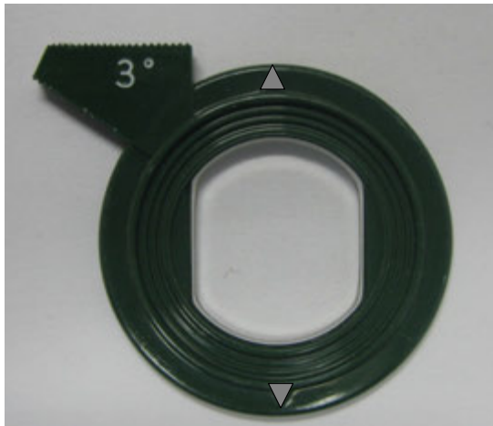
Figure 8.7: Plastic rimmed prism trial lens. This lens is a 3 rd prism. It is thinner at the apex of the prism, and thicker at its base.
